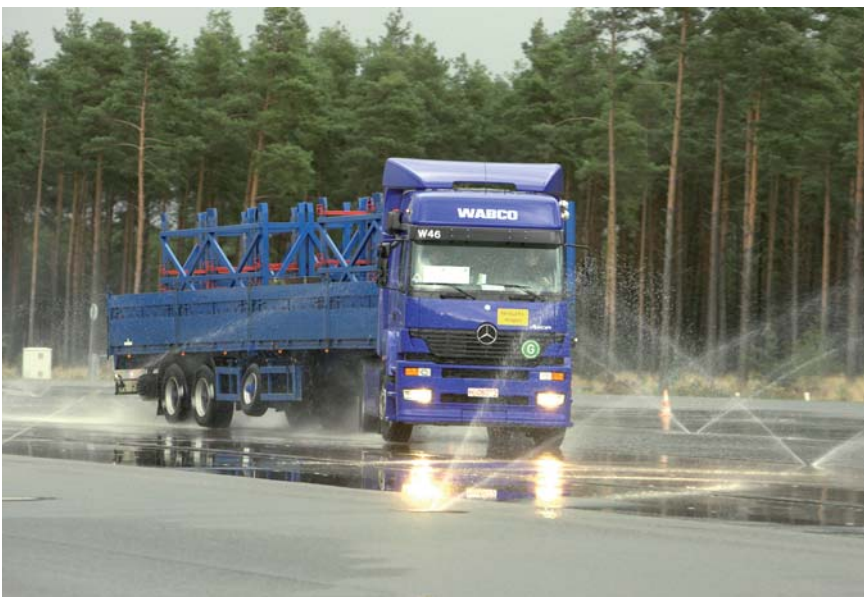
3 Test drive with ESC at the Wabco test track in Jevern (Germany)
