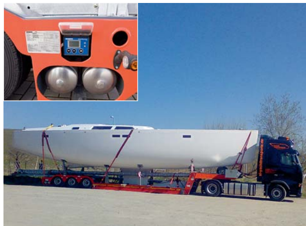
The boat trailer is equipped with the full WABCO Premium Trailer EBS E
