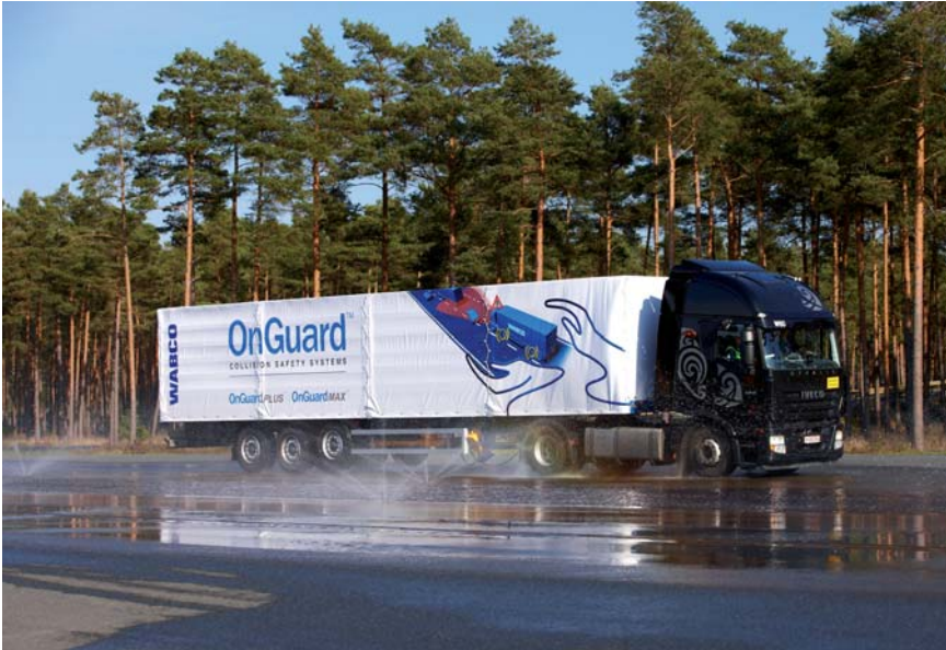
2 Test drive with ABS at the Wabco test track in Jevern (Germany)
